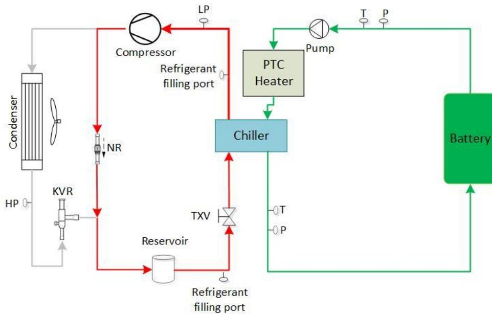
Figure 11 Architecture of Thermal Management System
