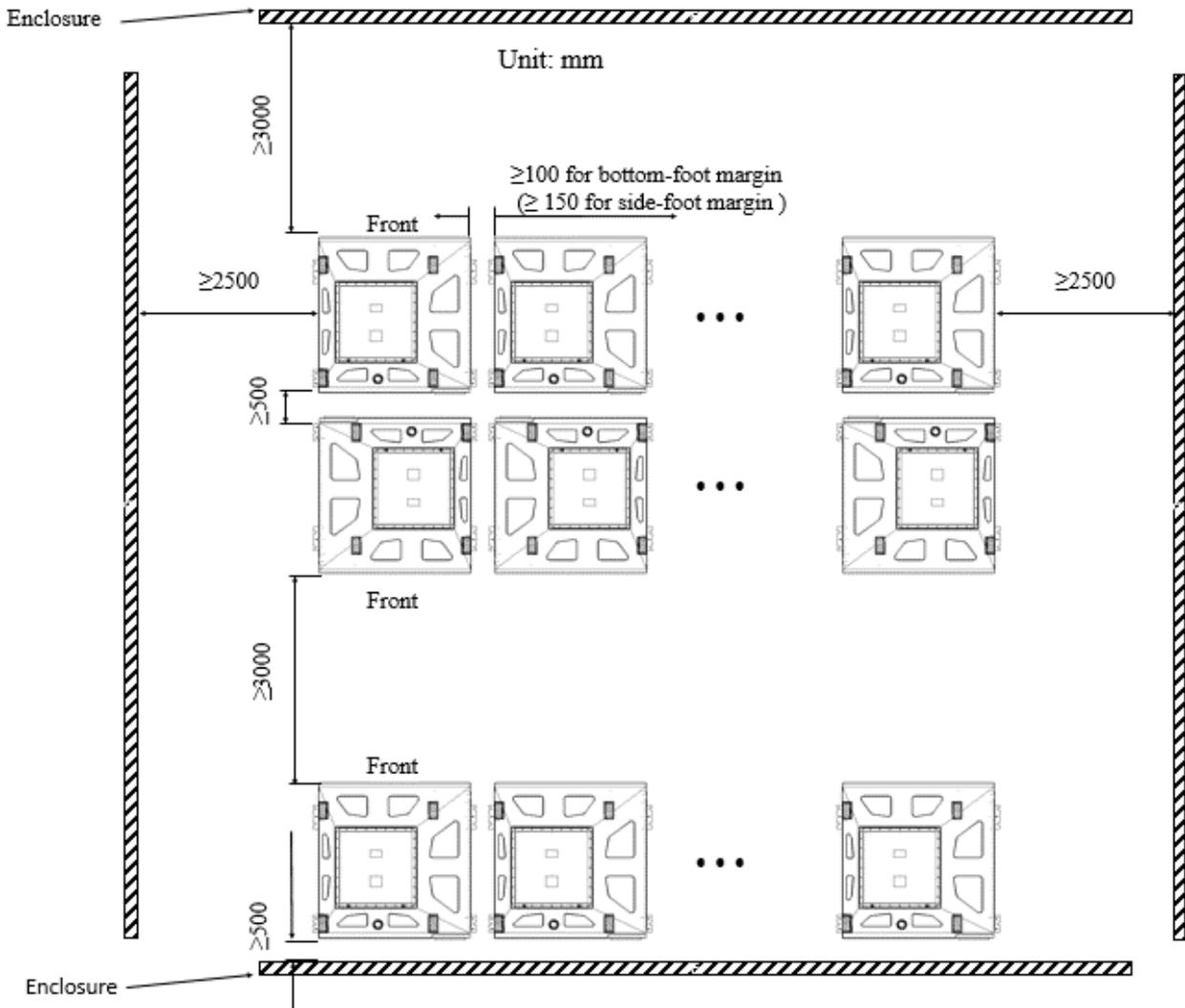
Figure 13 Layout of the rack
