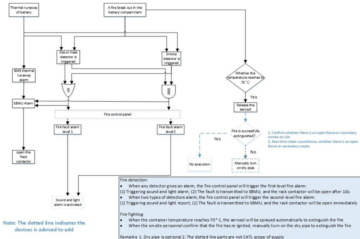
Figure 6 Control logic of FSS
