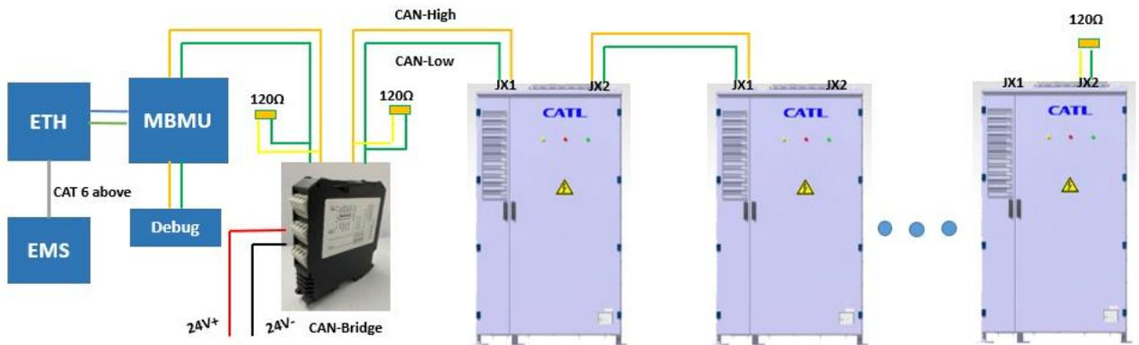
Figure 5 The Communication Architecture of the System
