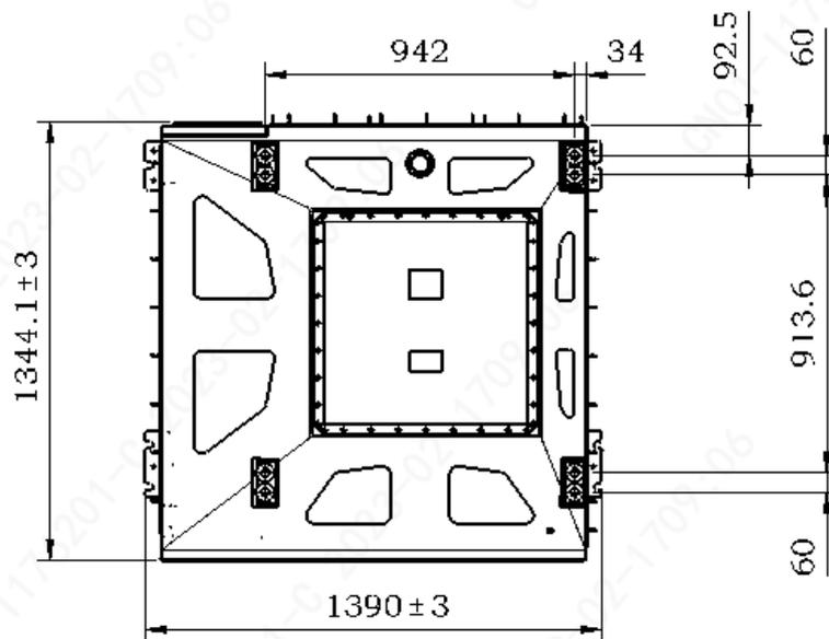
Figure 17 The Top View and Dimensions of EnerOne+
