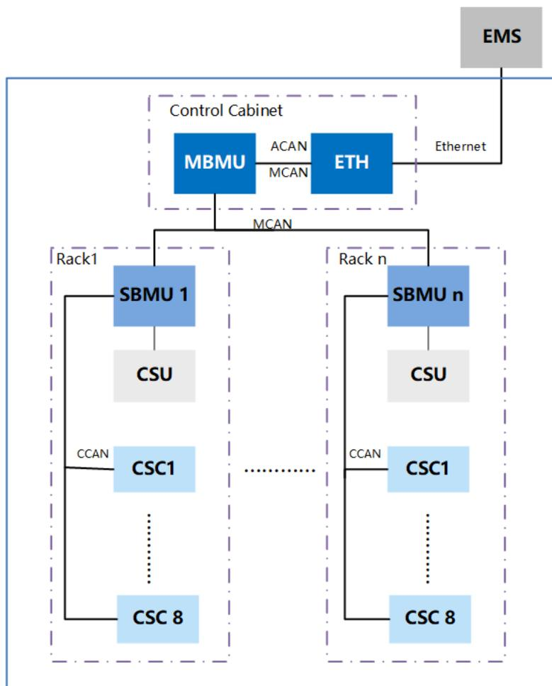
Figure 4 Three-Level BMS Architecture for n Racks in Parallel
